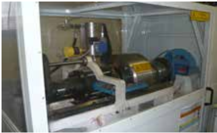
Test bench for slurry applications
